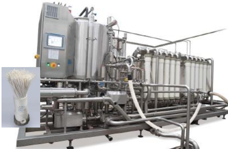
Filter skid (cut-away of a filter module inset)
